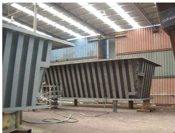
Stockpile Hopper Bin at Fabricators Works
